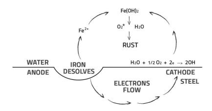
The rate of rust formation rapidly increases if the transfer of electrons from the anode to the cathode can be made easier; which happens if the conductivity of the water increases. This can occur due to the presence of dissolved salts, such as sea salts, on the surface or sulfur products from pollution fallout.
